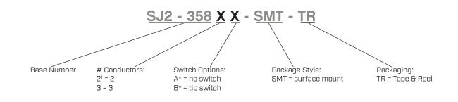
Notes: 1. 2 conductor option only available with tip switch \*Discontinued models SJ2-3583B-SMT-TR, SJ2-3583A-SMT-TR & SJ2-3582B-SMT-TR
