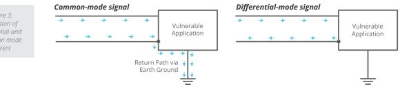
Figure 3: Definition of differential and common mode current
