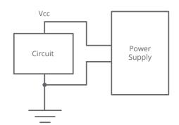
If there are multiple circuits in a system, decouple the circuits from each other by running separate supply lines, and/or place inductance in the supply lines as highlighted in figure 8 below.
